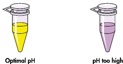
Figure 3. Indicator enables easy checking of the optimal pH. Indicator dye in solubilization and binding buffers (Buffer QG and Buffer PB) identifies optimal pH for DNA binding.
